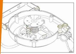
All the cable reels – up to a cable section of 3Gx2.5mm² - are supplied with **thermal protection switches**, which are triggered in case of overloading of the electric circuit.
