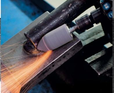
Abrasive shaft-mounted wheels Shaft Ø 6 x 40 mm
