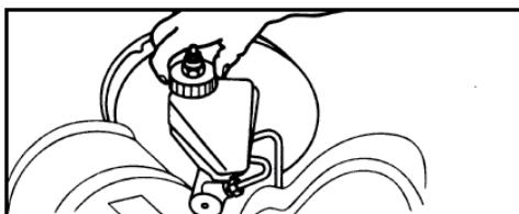
(see Adapter List) according to the instructions on the brake fluid reservoir.
