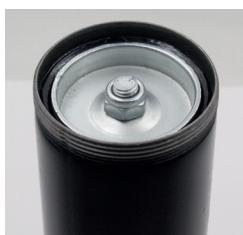
Depending on oil viscosity, adjust the nut on the plunger head (see picture): loose with particularly dense fluids; tight with less dense fluids.
