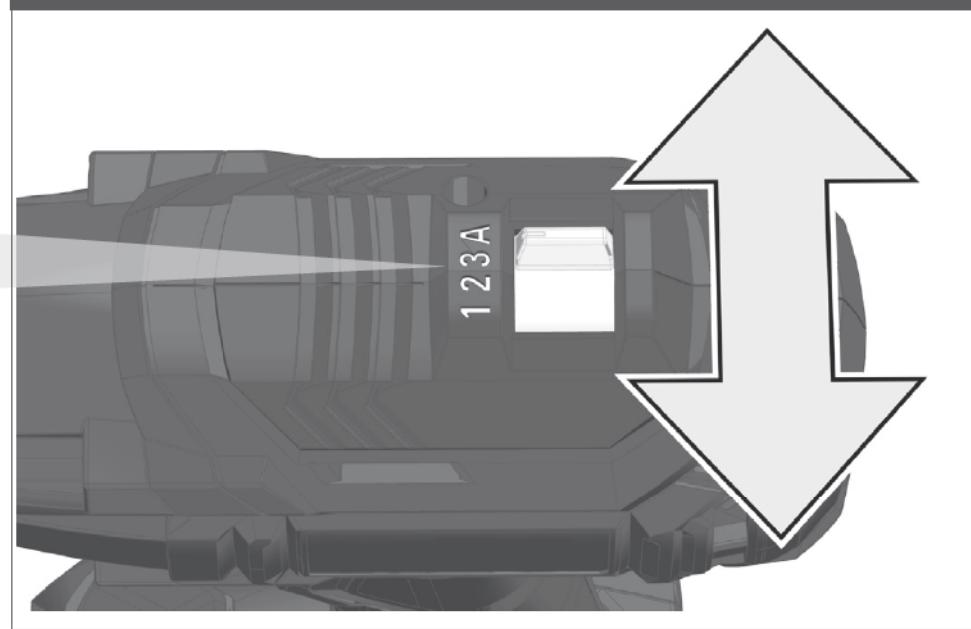
The "A" function is designed to give the user greater control in application and reduce damage to the fastener or work surface by automatically shutting the tool off after the tool senses the mechanism impacting for approximately one second.
