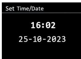
As for setting the hours and minutes, scroll through the numbers with the "TUNE +/TUNE -" buttons and press the dial to select the desired value. Then move on to the next value to be set. Once the last value has been set, the display will confirm that the new date and time have been saved.
