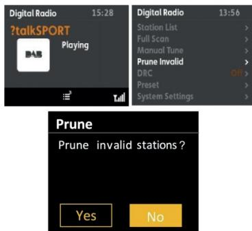
After selecting the station you wish to remove, select 'Prune'. from the MENU options. A choice of 'Yes' or 'No' will be presented. Select 'Yes' to remove the station. Use the Tune+/- buttons to scroll through the options and press the wheel to confirm.
