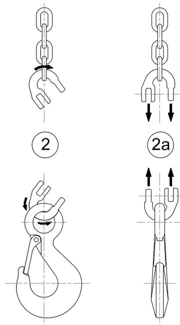
Fit the hook system of the part to lift into the hook housing, pushing the mouth closing device inwards; such device will be automatically restored to the closing position after it has been fitted in, being pushed by the spring.
