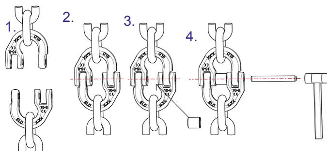
1. by introducing the two half connecting links into the end of the chain (or other linking element)
