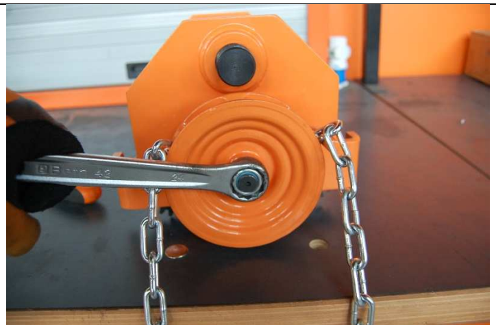
Unscrew the nut that lock the operating wheel.
