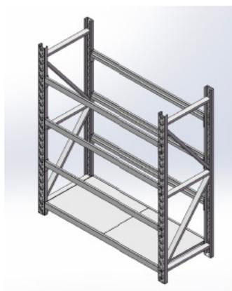
4. Put the shelf on the beams as shown in picture, from bottom to top
