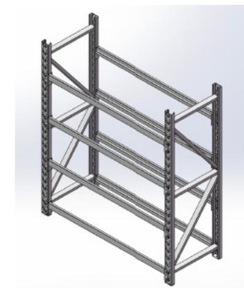
3. In a similar way install the other beams and safety-pins
